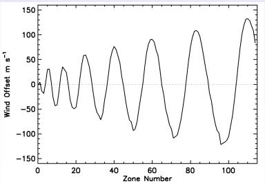
Averaging uncorrected "Doppler shifts" over a large number of dense-cloud sky observations produces the required velocity offset correction for each zone. The characteristic signature seen here arises because the zones "spiral" out from the center with increasing index number.
