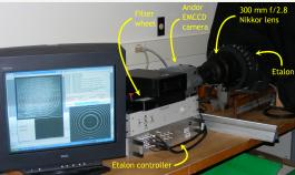
The first thing to do to control chromatic aberration is to use a high quality lens to form the fringe images.
