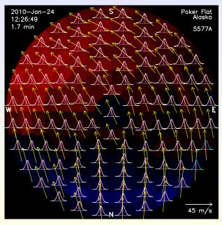
This is an example of a Doppler sky map after zero velocity correction, along with the 2-dimensional horizontal vector wind field that was fitted to it.
