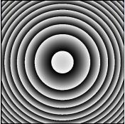
In a conventional imaging FPS, correction for the etalon-induced chromatic aberration would amount to finding the fringe center at 558nm. This would normally be determined using calibration fringes, but here of course it must be done using sky fringes – or with an averaging procedure using a large number of sky fringes.
